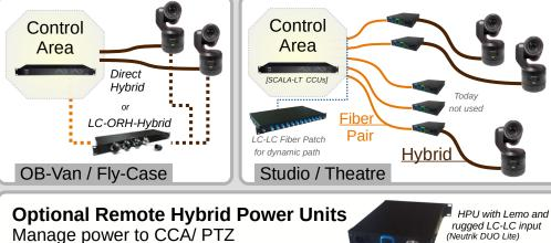
**1RH Wall Box / SHED (½RH)** Single Channel Hybrid Interface **ORH Unit** Host up to 4Ch Hybrid Interface (1RU) HPU with Lemo and rugged LC-LC input (Neutrik DUO Lite)
